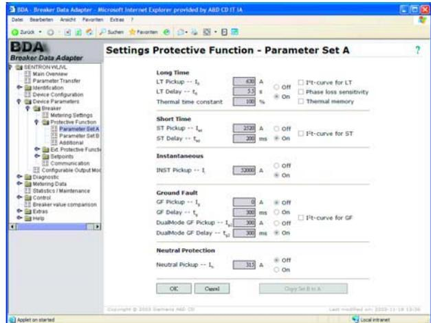
Breaker Data Adapter – device parameters
